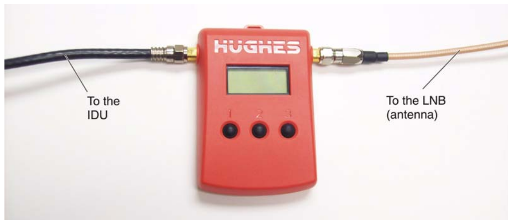
Figure 7: Installing the DAPT
